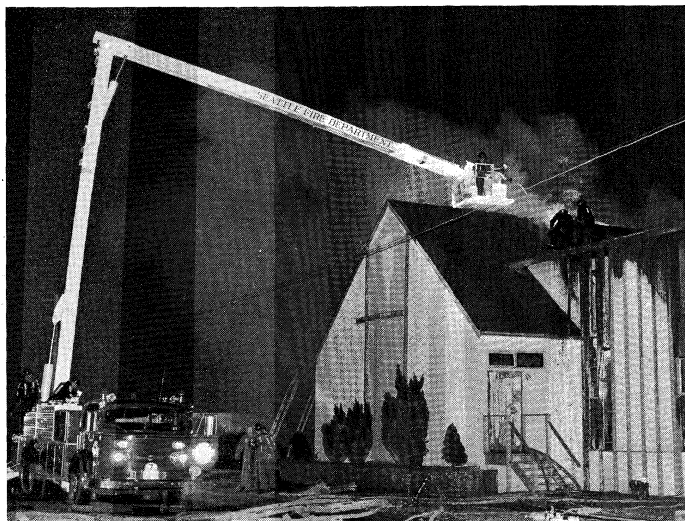
Figure 2: Elevated-platform fire apparatus, known as a snorkel, consisting of a hydraulically operated boom attached to a truck-mounted turntable and equipped with a turret nozzle.
