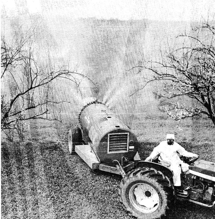
Figure 2: Air-concentrate mist blower used to spray bush fruits, grapes, and compact high-density tree fruits.
